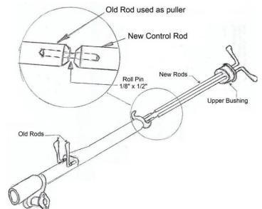
This worked really well aligning both rods through the correct holes during installation. I put my steering column in a vise in the horizontal position and used wood blocks to support the new rods so their entire weight wasn't hanging on the roll pins. The roll pin, also known as a split pin a spring pin or tension pin, is available at your local hardware store.
