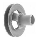
The problem with the one-piece pulley is it's impossible to replace one with the radiator installed, and not that easy with it removed. With the pulley being really close to the frame, the front of the engine usually must be raised to remove it.
