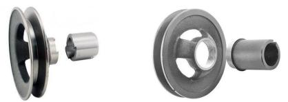
A newer two-piece design has a threaded (left hand thread) connection. These work much better, will stand up to a load, and can be serviced with the engine in the car.
