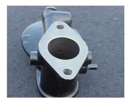
The small hole in the throat of the upper casting allows air to flow into the idle circuit when the throttle is closed.
